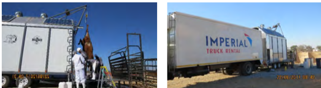
Figure 12. Mobile abattoir unit with associated stunning crush and refrigerated truck for transportation of carcasses.
